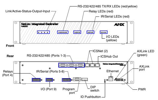
FIG. 2 NI-2000 front and rear panel components
